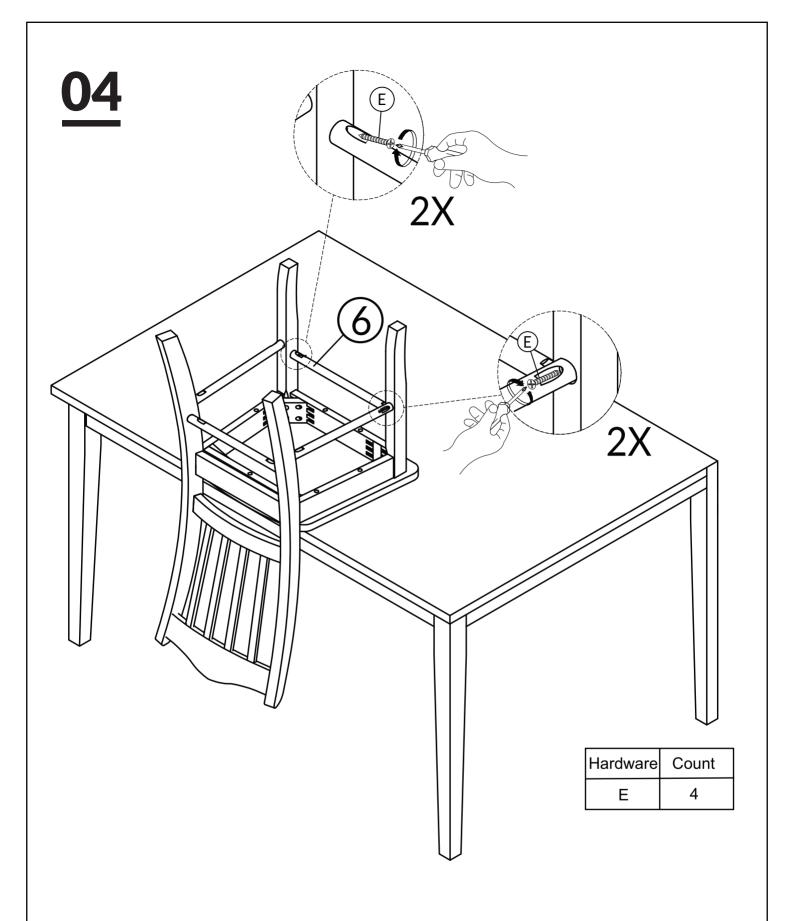
TIGHTEN BOLT AND SCREW COMPLETELY.
