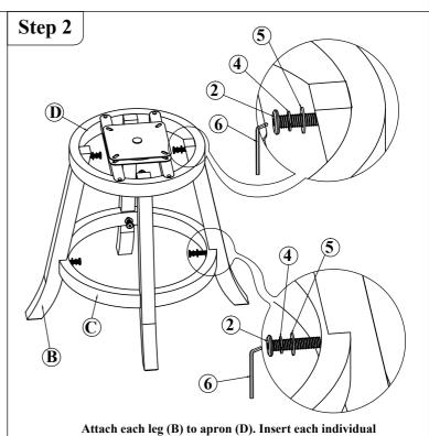
hardware as show in the picture. Then tighten the 4 legs with apron first, then tighten the footrest with the 4 legs completely.
