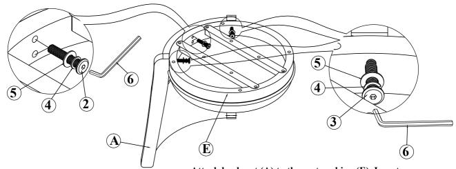
Attach backrest (A) to the seat cushion (E). Insert 6 sets of hardware as shown in the picture. Tighten together after alignment is done.
