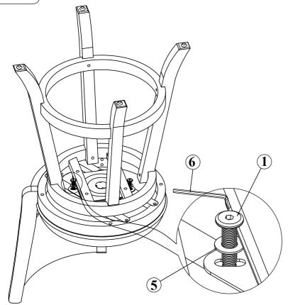
Attach the assembled base from step 2 to the assembled top from Step 3. Insert 4 sets of hardware as shown in the picture. Tighten together after alignment is done.
